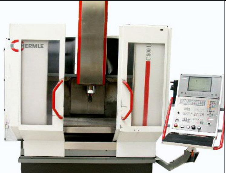
A photograph of a Hermle C800U 5-axis CNC milling machine. It features a white and red design with two vertical columns and a horizontal base. The model number 'C 800 U' is on the side. A control unit with a screen and keypad is located to the right. |        | <p><b>Baujahr</b><br/>2005</p> <p><b>Steuerung</b><br/>Heidenhain</p> <p><b>Arbeitsbereich</b><br/><b>X</b> 800 mm   <b>Y</b> 600 mm   <b>Z</b> 500 mm</p> |
