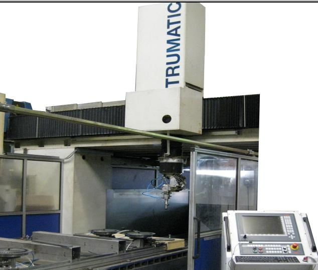
A large industrial machine with a vertical column labeled "TRUMATIC". It features a robotic arm with a torch or cutting head at the end, positioned above a worktable. A control cabinet with a touchscreen monitor is located to the right of the machine. | <p><b>Baujahr</b></p> <p><b>Steuerung / Leistung</b><br/>IBH / 2,5 KW</p> <p><b>Verfahrwege</b><br/>X 3000 mm Y 1300 mm</p> <p><b>Material</b><br/>ST, VA,</p> |
