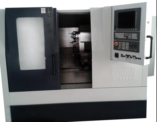
A black and white Spinner TC600 65 MC CNC lathe with its door open, showing the internal structure, and a control panel with a touchscreen and buttons. | <b>Baujahr</b><br>2011<br><br><b>Steuerung</b><br>Siemens<br><br><b>Arbeitsbereich</b><br>X 500 mm Y 150 mm Z 700 mm   |
