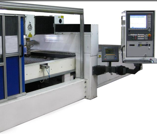
A large industrial machine with a horizontal worktable and a control cabinet featuring two monitors. The machine is enclosed in a metal frame with blue panels. | <p><b>Baujahr</b><br/>2003</p> <p><b>Steuerung / Leistung</b><br/>IBH / 2,5 KW</p> <p><b>Verfahrwege</b><br/>X 3000 mm Y 1500 mm</p> <p><b>Material</b><br/>ST 12 mm VA 6mm</p> |
