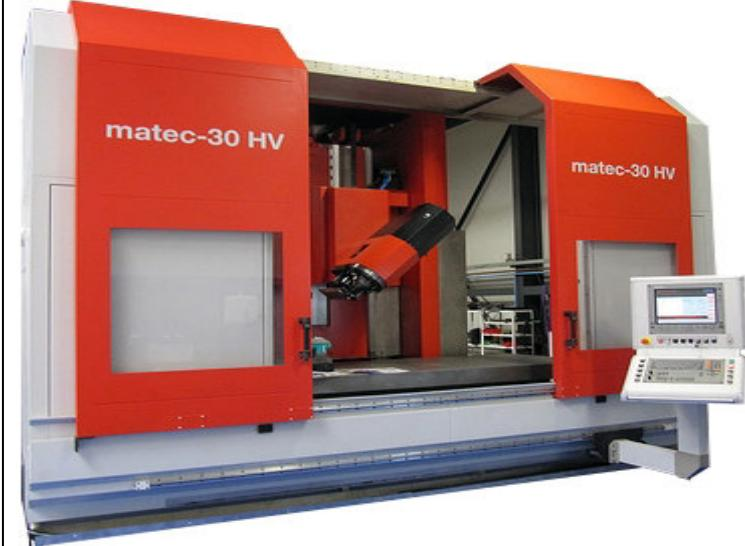
A red Matec 30HV CNC milling machine with a large horizontal worktable. The machine features a central vertical column and a horizontal bridge-style gantry. A control panel is located on the right side of the machine. | <p><b>Baujahr</b><br/>2000</p> <p><b>Steuerung</b><br/>Heidenhain</p> <p><b>Arbeitsbereich</b><br/><b>X</b> 3000 mm <b>Y</b> 800 mm <b>Z</b> 800 mm</p> |
