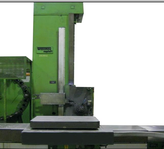
A vertical drilling machine with a green cabinet and a silver vertical column. The model number 'WOTAN rapid 26104' is visible on the cabinet. The machine is mounted on a grey base plate. | <p><b>Baujahr</b><br/>1980 – Modernisierung: 2008</p> <p><b>Steuerung</b><br/>Heidenhain</p> <p><b>Arbeitsbereich</b><br/><b>X</b> 1600 mm   <b>Y</b> 1600 mm   <b>Z</b> 1000 mm<br/><b>W</b> 600 mm   <b>B</b> 360°</p> |
