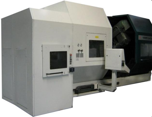
A white Monforts UniCen 1000 CNC lathe with a control cabinet and a workpiece being machined.                                                            | <b>Baujahr</b><br>2001<br><br><b>Steuerung</b><br>Siemens<br><br><b>Arbeitsbereich</b><br>X 1000 mm Y 200 mm Z 1000 mm |
