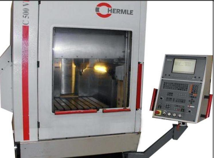
A photograph of a Hermle C500V CNC milling machine. It is a vertical mill with a grey and red finish. The model number 'C 500 V' is visible on the side panel. A control unit with a screen and keypad is positioned to the right of the machine. | <p><b>Baujahr</b><br/>2005</p> <p><b>Steuerung</b><br/>Heidenhain</p> <p><b>Arbeitsbereich</b><br/><b>X</b> 400 mm   <b>Y</b> 500 mm   <b>Z</b> 450 mm</p> |
